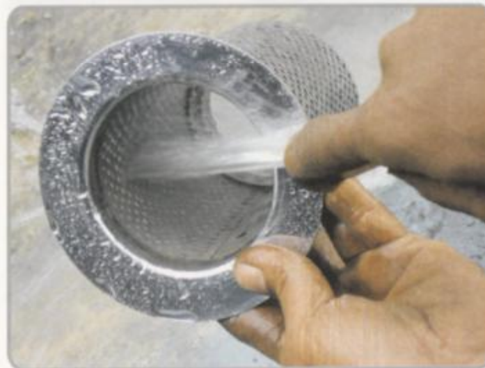
2. Wash the filter with a Garden hose pipe or under the tap.
