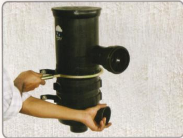
8. Tighten the Union using special Tool.
