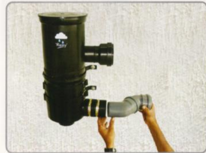
1. Insert Rubber bush with suitable P.V.C. pipes to the clean water outlet of the filter & tighten the hose clamps.
