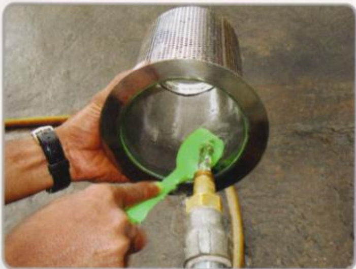
10. The steel filter element can be washed through garden hosepipe / tap water by using a brush incase the filter is fully choked.
